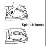
Please check carefully. The laundries may fall to the lower part of the outer side of the spin tub (as indicated in the figure).
